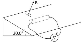
To keep the metal from rolling down the incline, an adjustable voltage source is attached to the ends of the wire. When the correct amount of current flows through the metal it remains at rest.
